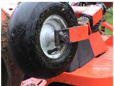
On the other end of the axle I fitted a plate to the axle which picks up the original axle safety pin retaining bolt hole in the yolk and secured it with a bolt and stiff-nut. This mod has reduced the daily "before use" servicing time, significantly reduced bearing replacement costs and restored the original height setting as well as eliminating all slop and wear areas.
