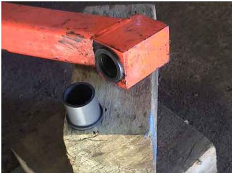
I replaced the jockey wheel roller bearings and stem bushes with "X-Lube" plastic bushes, The plastic bush cost about \$2 each and dont require greasing. (a little on assembly stops squeeking).
