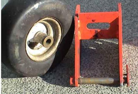
On the Jockey wheels, I was not happy how the yolk holes flogged out, wore out the axles and lost consistant deck height. I devised a mod which is more rigid and maintains accurate height. I made up new 3/4" axles with a UNF thread on the end & welded a nut on one leg of the yolk.
